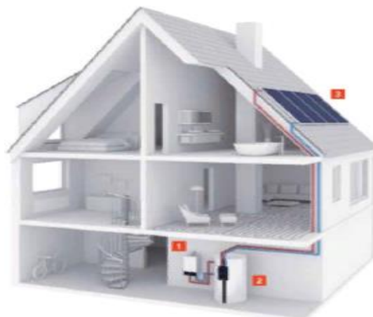
Figure 3 - The location of the elements of the solar heating system 1 - condensing boiler; 2 - combined tank for water and maintaining of heating system; 3 - flat plate solar collectors
