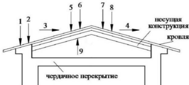
Figure 1 - Impacts on the roof
