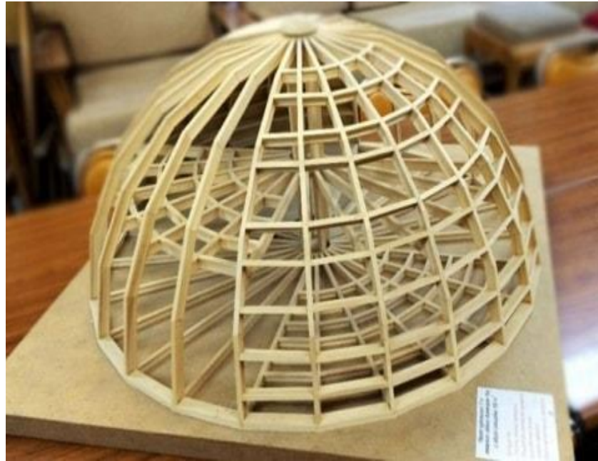
Fig. 2. Frame of a domed house without a single nail
