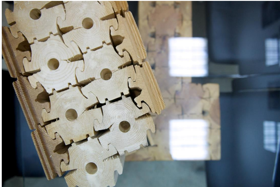
Fig. 1. Structural sheets from thin tree trunks
