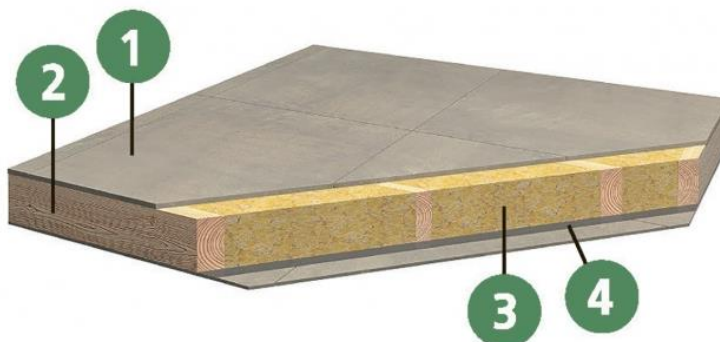
Fig. 3. Floor and attic roof panels
