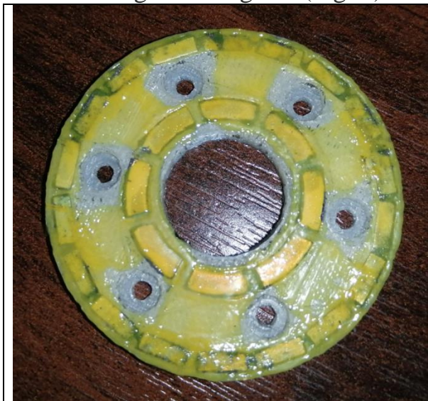
Fig. 3. Magnetic ring of a prototype encoder
