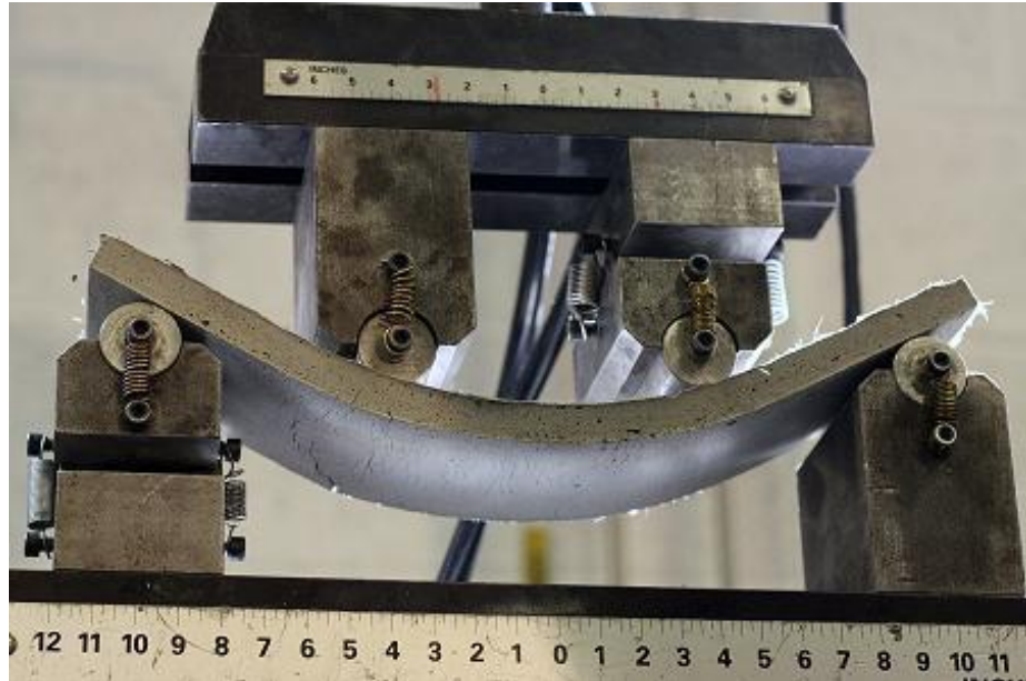
Fig. 6. Strength test under load after self-healing
