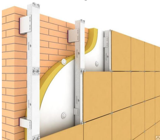
Fig. 2. Thermal insulation of external walls before thermal modernization
